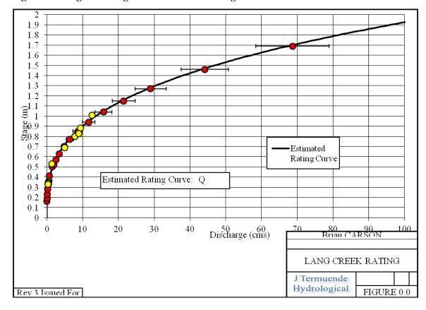
Figure 13. Stage Discharge Curve for Lower Lang Creek
